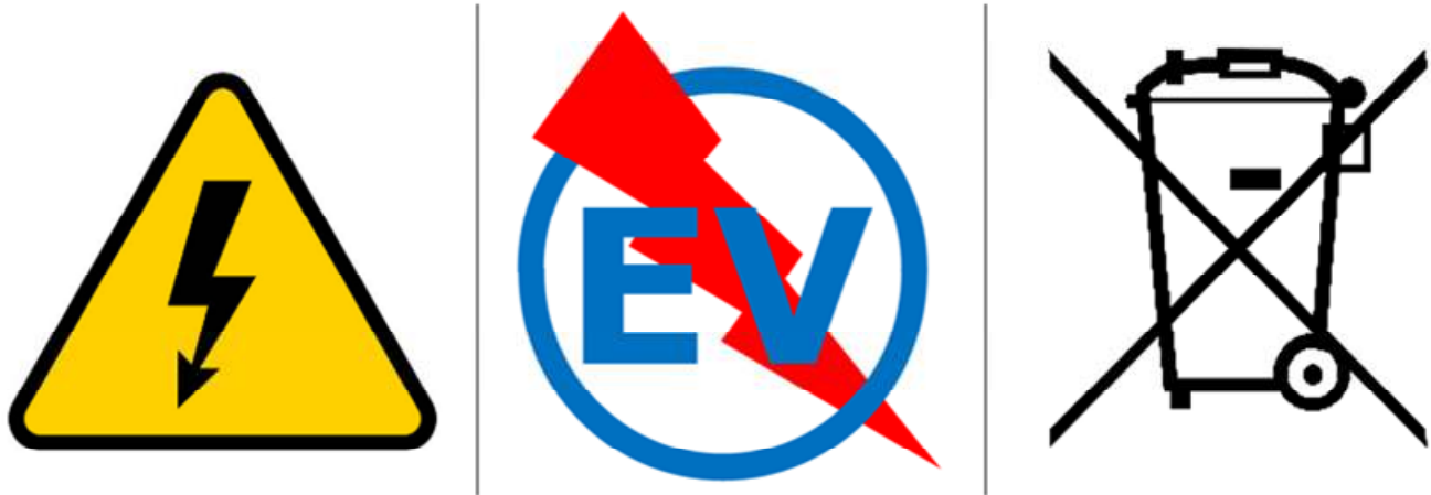
Figure 2 : A few required labels: Electric Vehicle Sticker, “High Voltage” (>60V), and non-disposable (battery). EV sticker size varies by vehicle class.
