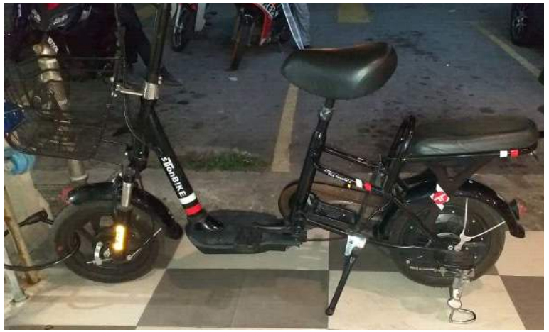
Figure 36 : Electric bicycle parked in Bandar Saujana Putra, Malaysia. Note the chained front wheel and missing battery (large open slot in frame behind seat post).
